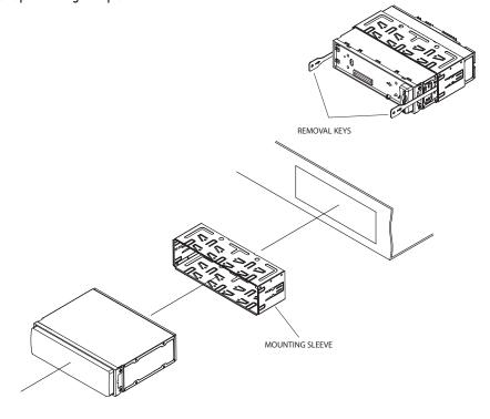
TYPICAL FRONT-LOAD DIN MOUNTING METHOD
